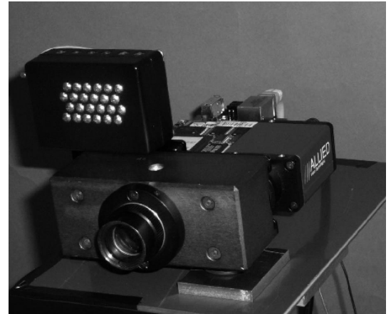
Figure 2: 2D/3D camera setup with PMD, RF modulated optical source, CCD and the Image Multiplier
