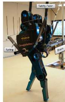
Figure 1: (a) The planar (2D) biped MABEL was developed for the study of highly dynamic locomotion. (b) High-level motion primitives in MABEL to allow walking over very rough ground without tripping. While tools for automatic low-level control algorithm synthesis are well developed, at the state machine level, all tuning was done by hand for lack of appropriate tools. “Probable correctness” was established through extensive simulation and experiments.
