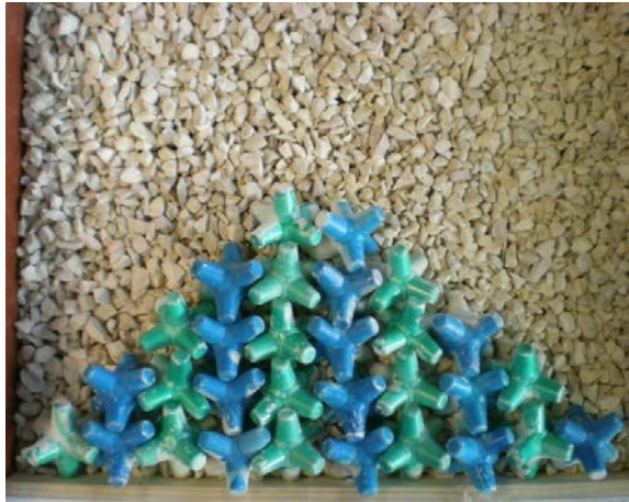
Uniform placement using smaller underlayer in a rectangular grid
