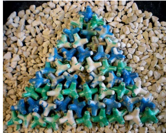
Random placement using conventional underlayer in a diamond-shaped grid
