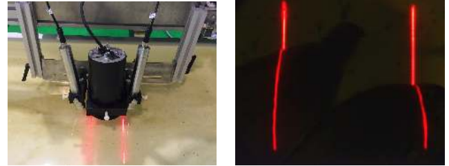
(a) Structured Light Vision System - Camera and red lasers. (b) Snapshot Structured Light Vision Image, red laser line deformation in the presence of a fish.
