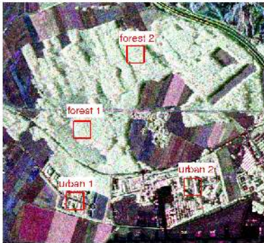
Fig. 6. 2 forest areas and 2 urban areas (30x30 pixels) are selected into the Oberpfaffenhofen image.
