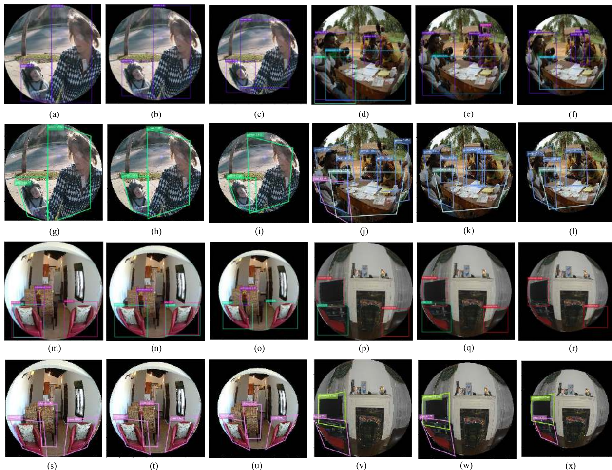
FIGURE 11. Baseline vs the proposed FisheyeDet. The first and third lines images are based on the baseline for detecting objects and locating the objects under different distortions. The second and last line images are based on the FisheyeDet for detecting objects and locating the objects under different distortions.
