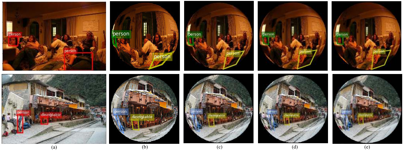
FIGURE 9. Representative samples of the VOC-Fisheye dataset. (a) original images from the PASCAL VOC [23], (b),(c),(d) and (e) fisheye images with different distortions.
