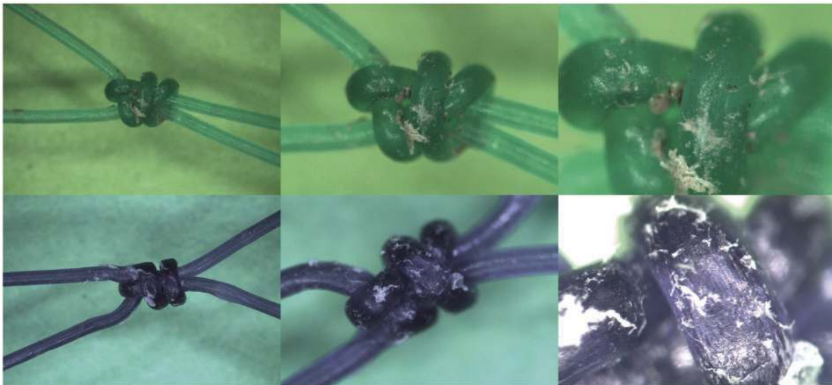
Figure 4. Images of the bio gillnets from 2016 (green) and 2017 (blue) showing physical damage of the knots.
