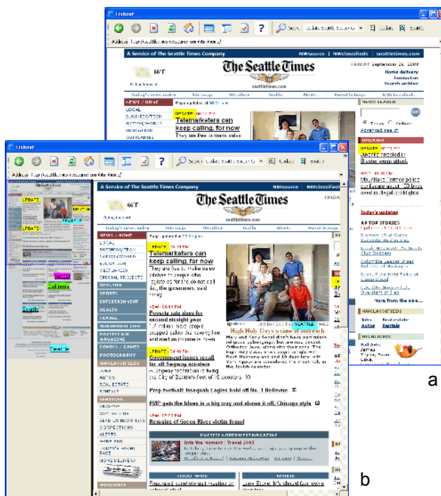
Figure 1: (a) Displaying a long web page in a regular web browser results in page content being clipped. (b) Showing clipped content using an overview enhanced with popouts (similar to [27]).
