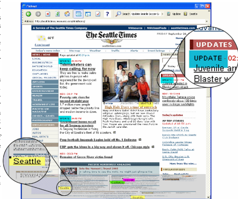
Figure 2: The fishnet web browser fits web pages of any length into the browser window by vertically compressing peripheral content. Color-coded popouts keep search terms ('Seattle', 'update', ...) readable while they are in one of the context areas.
