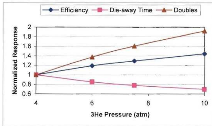
Fig. 2. Simulated efficiency and die-away times as a function of ^3\text{He} gas pressure for a 25.4-mm-diameter tube with normalization at 4 atm gas pressure.
