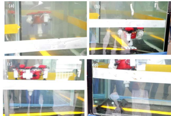
Figure 9. Control system experiment result (a) forward and reverse (b) down (c) left & right (d) up
