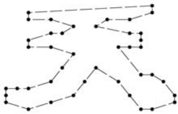
(c) 42 control points of an initial B-spline curve.
