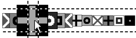
Fig. 11. If targets are tiled along one dimension, and expansion depends only on the current cursor position, expansion in motor space is only possible along the other dimension. Dashed lines delimit the footprint of a button in motor space. The cursor must be within this rectangle to acquire the button. Although the button looks larger than this rectangle in visual space, its full visual size is not available to the user: as soon as the cursor moves off the button's centre, the button begins to contract. The rectangle in motor space is in fact no wider than the unexpanded button, however it is taller, which should ease selection somewhat if the cursor approaches from above or below [Accot and Zhai 2003].
