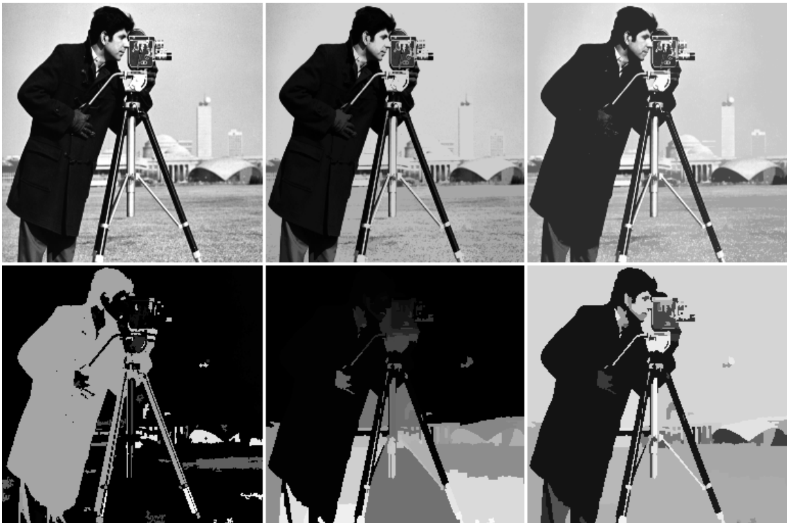
Figure 10: Contrast-oriented segmentation. First row: original image, simplified image (positive contrast), and simplified image (negative contrast). Second row: markers, segmented regions and segmentation results.
