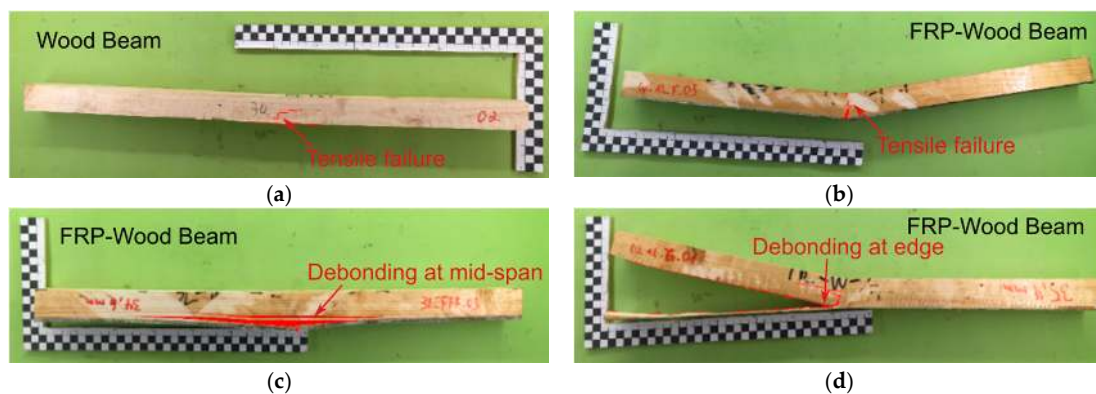
Figure 5. Typical failure modes of FRP–wood beams under three-point bending with different FRP laminates: (a) tensile failure for reference wood beam, (b) tensile failure (W_1L-F), (c) debonding at mid-span (W_3L-F) and (d) debonding at edge for FRP strengthened wood beam (W_1L-G).
