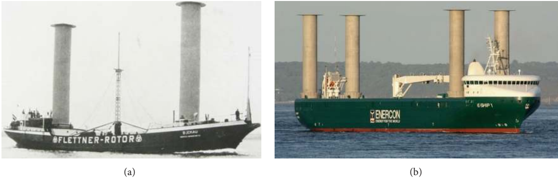
FIGURE 1: Buckau, first Flettner's ship (a), and E-Ship 1 by Enercon wind company (b).
