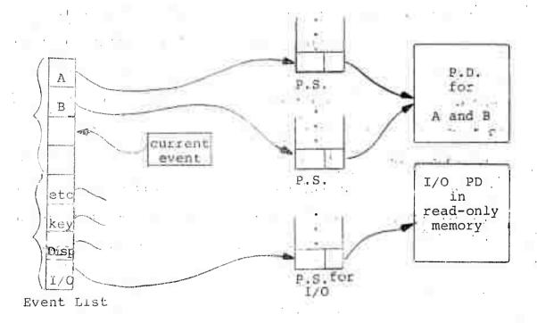
All the real-time event notices are logically clustered. Between each event they are scanned by the scheduler to see if activation is required. If not, the process pointed to by the current-event pointer is activated. At any time an outside interrupt may point into the real-time area. When this happens, the current event is passivated and the real-time event activated.
