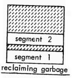
There are several ways to remap segments. The cheapest is to find a large enough area of garbage and reallocate the segment. If this cannot be done, then garbage must be collected and arranged to form a large contiguous free space which may then be used for allocation and new segment creation.
