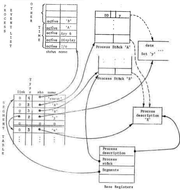
The dotted lines are effective pointer (meaning that the reference really has ta go through the segment rable. An event for 'A' is taking place as shown by the base register configuration.
