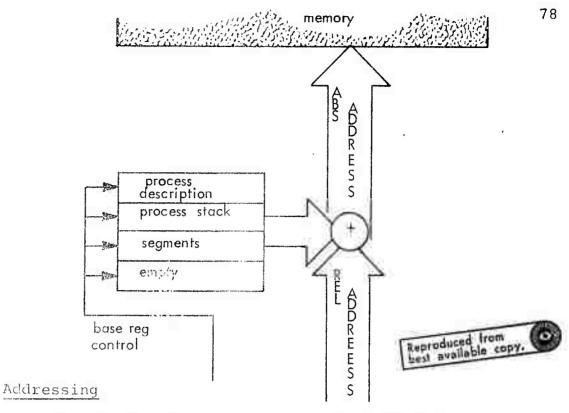
It can be seen that although the FLEX environment has effectively done away with direct addressing and introduced relative (and moveable) data entities in the segmenting scheme, takings actually hold still for the major part of the time and the basic overhead during an event is a short add whose time will be absorbed by the micro code hardware.
