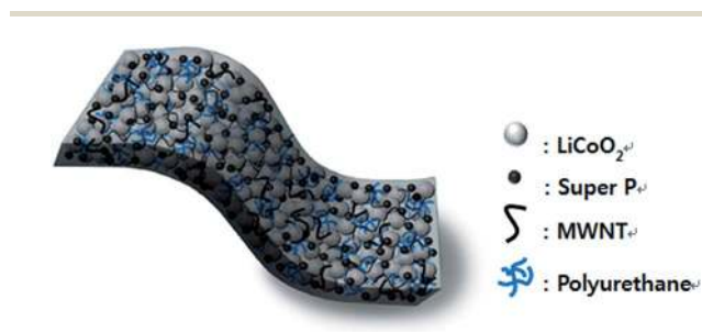
Fig. 1 Schematic of a free-standing electrode comprising LiCoO 2 , Super P, MWNT, and polyurethane.
