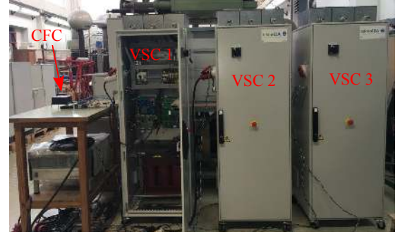
Figure 16. Scheme of the experimental 3-terminal meshed DC grid with a 3-port CFC in the laboratory.
