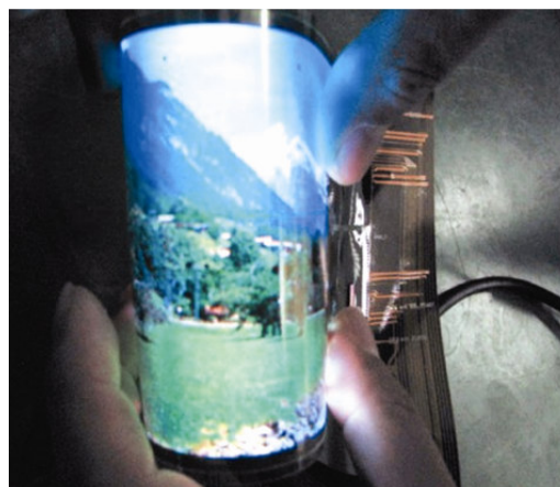
Fig. 8—Flexible OLED display (0.05 mm) by Samsung
