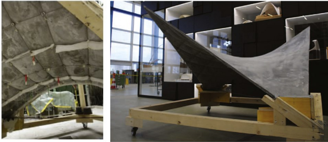
348 Figure 12 – Hybrid cable net and fabric formed shell Photo: Block Research Group, ETH Zurich [45].
