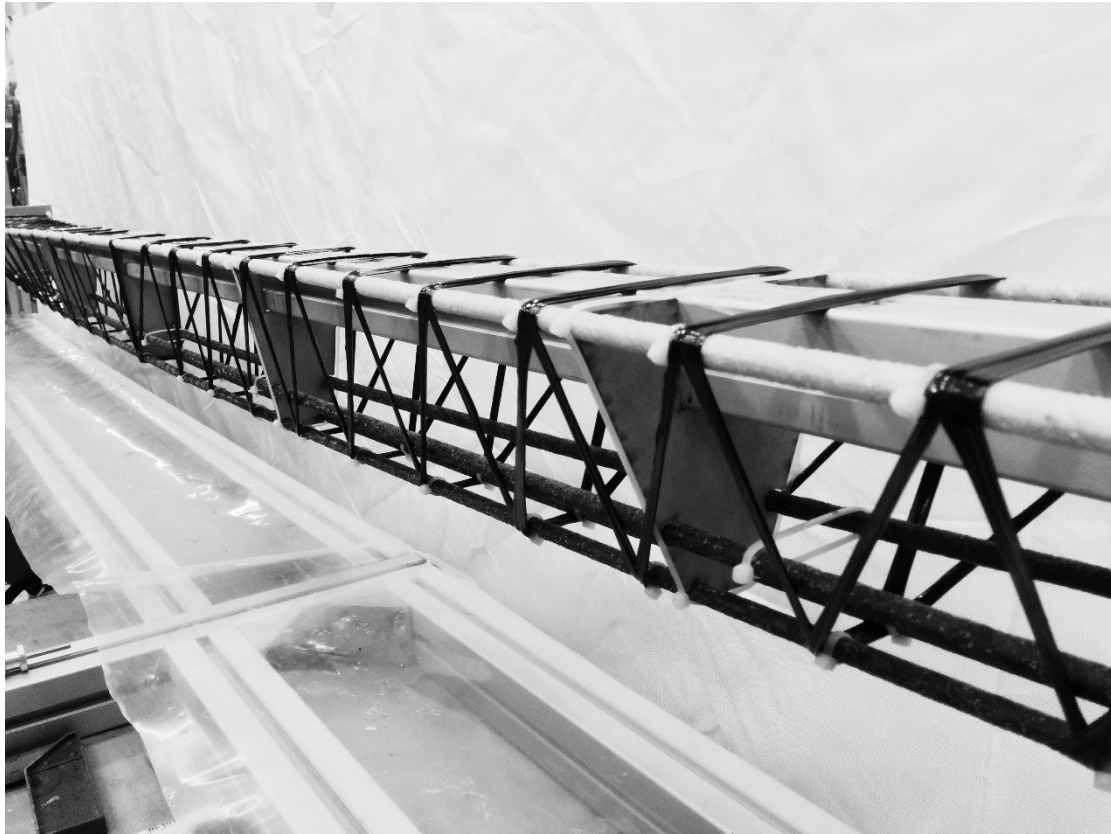
Figure 20 – Bespoke carbon fibre reinforcement for non-prismatic beams. Photo: John Orr.
