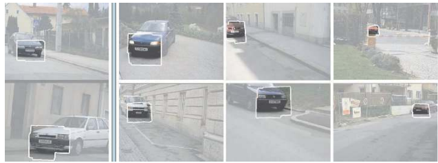
Figure 2. Left column: the two base images for a PSM; Right: a few validation matches for the same PSM. The outline of the PSM, defined as the union of matched feature regions, is shown in white.
