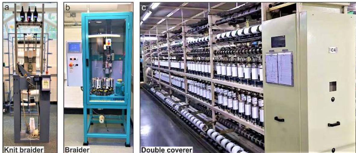
Figure 2. Industrial machines utilised for covering the flexible RTDs. (a) Rius MC/2 knit braider from RIUS-COMATEX used to create the knit braided yarn. (b) RU 1/24-80 braiding machine from Herzog ® utilised to fabricate the braided yarn. (c) Menegatto 1500 (Menegatto S.r.L) used to build the double covered yarn.
