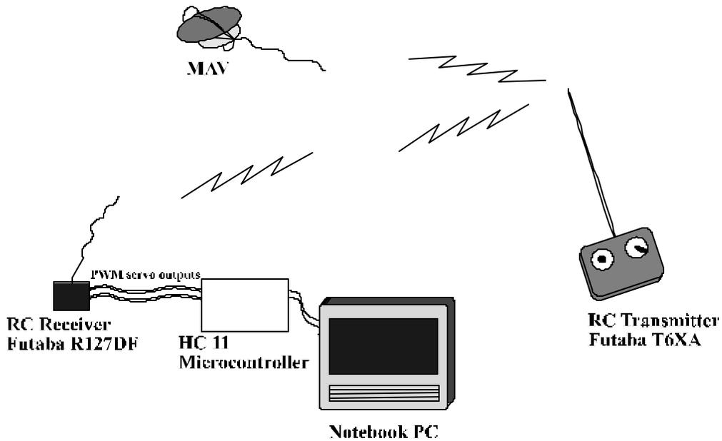
Figure 11. Flight control input data recording system.
