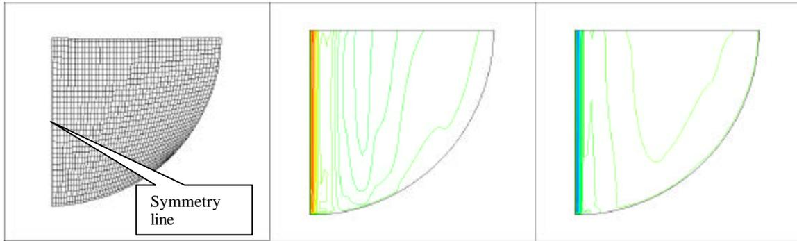
**Figure 6.** The schematic of the wing geometry, shown with representative grid layout for CFD simulations, and the pressure contours on upper and lower wing surfaces at angle of attack of  $6^\circ$ . The camber Reynolds number is  $6 \times 10^4$ .
