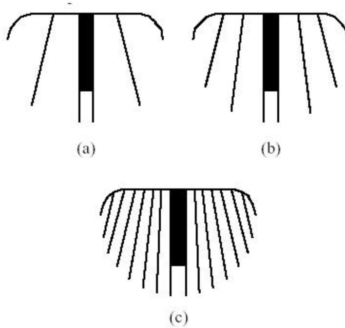
**Figure 8. Batten arrangement for membrane wings.**
