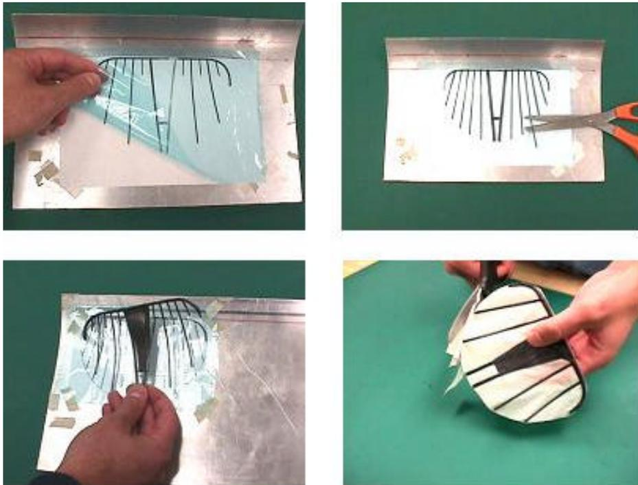
Figure 5. Illustration of the wing construction process.
