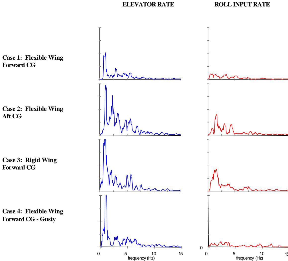
**Figure 12. Autospectra of elevator movement rate data and roll input rate data. The vertical axis is the relative power at each frequency. The curves are generated by processing the differentiated elevator and roll input data (512 data points each case).**
