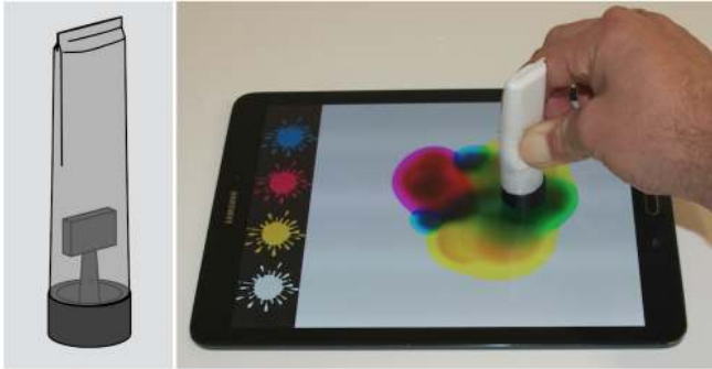
Figure 10. Mixing colors by squeezing them out of a deformable tube.
