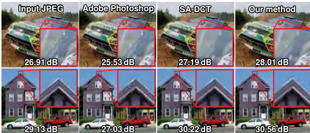
Figure 14: Extending the reconstruction pipeline to the receiver. We compare the JPEG (quality = 30), Adobe Photoshop deblocking, SA-DCT, and our reconstruction on the display side (PSNR in images). (Images courtesy of Wikipedia user kallerna, and A. Torralba & B. Russell / LabelMe dataset.)
