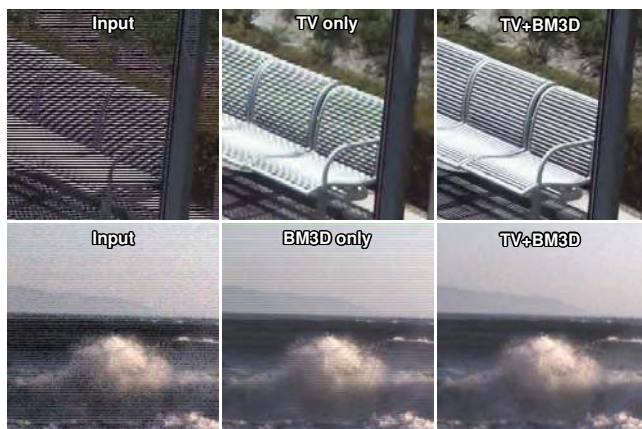
Figure 5: Illustration of using both the TV and BM3D priors for reconstructing images from the interlaced HDR sensor (Sec. 4.3).
