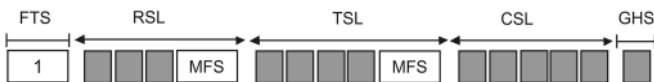
Fig. 2. A node's transmission schedule structure. The slots are not contiguous in time.
