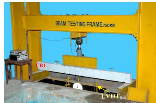
Fig. (4). Test Set Up for Static Loading.
