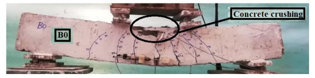
Figure 10. The final crack of beam B0-Control.
