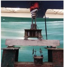
Figure 8. Test setup of RC beams.
