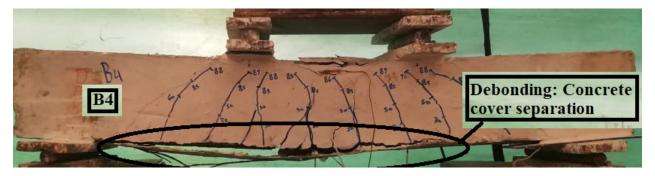
Figure 14. The final crack of beam B4-0-EP.
