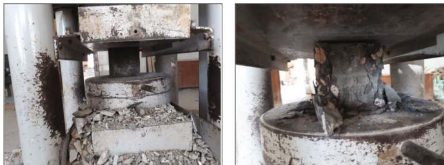
FIGURE 5: Hydraulic machine used in a compressive test and mode of a crushed cube.
