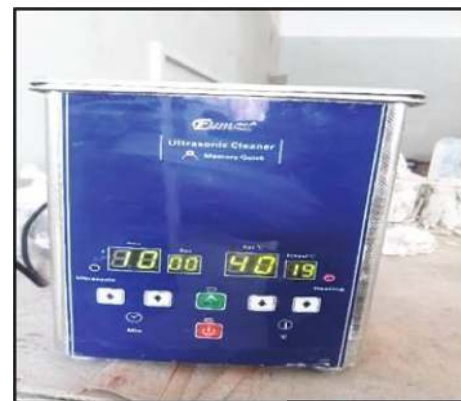
FIGURE 4: Ultrasonic device for mixing nanoparticles.
