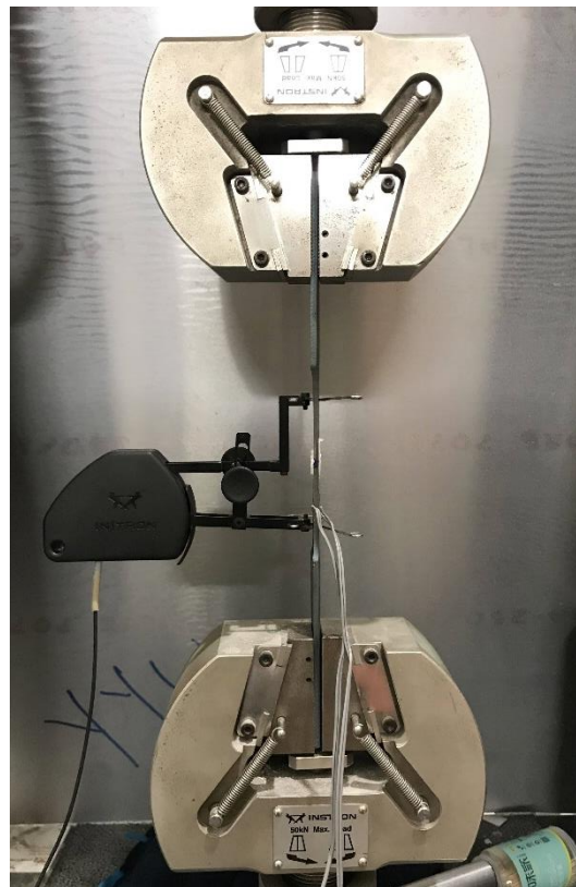
Fig. 4. Material tensile coupon test setup.
