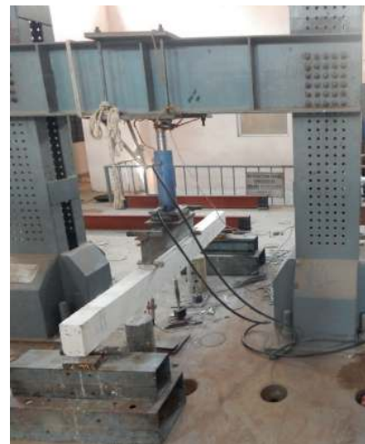
Fig. 5 Four point load test setup on beam
