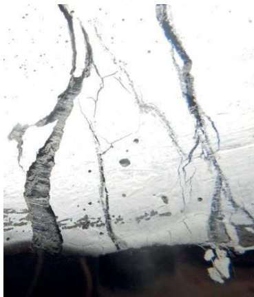
Fig. 15 Fiber bridging effects in ECC layer
