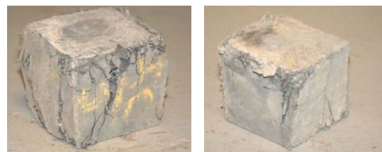
Fig. 7 Typical failure pattern of ECC cubes
