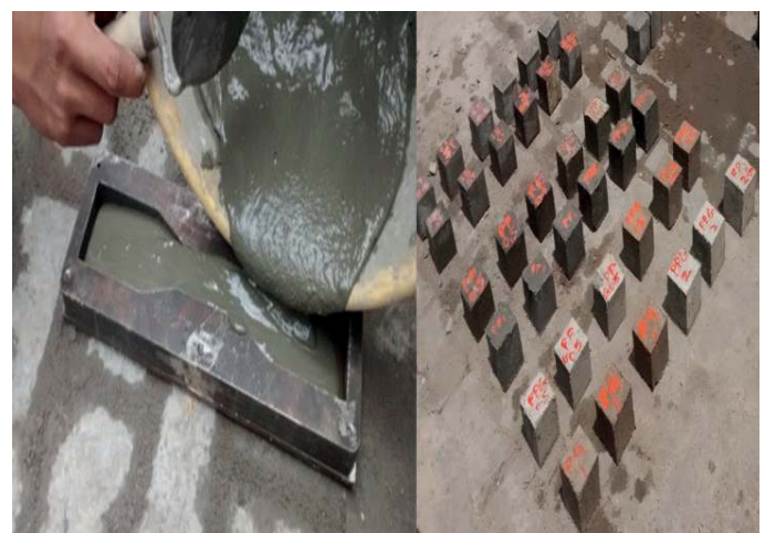
Fig. 1 Casting of dog bone specimen and cube specimen
