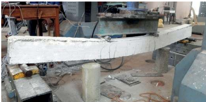
Fig. 13 Flexural behavior of ECC layered beam under ultimate loading
