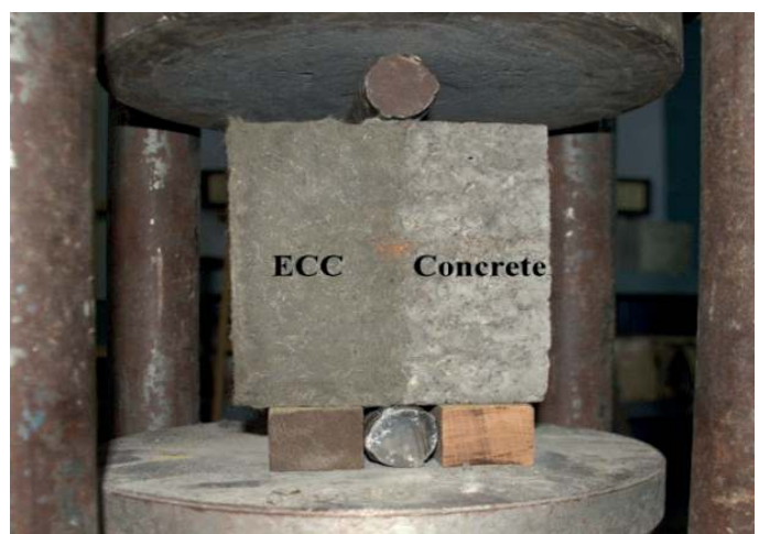
Fig. 3 Bond test on conventional concrete cube
