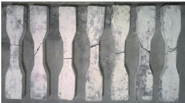
Fig. 10 Failure pattern of ECC specimen under direct tensile load
