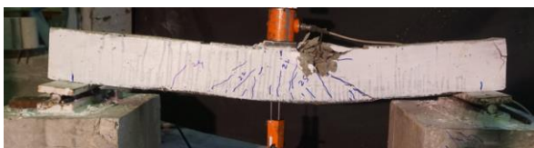
Fig. 9. Failure mode of beam JFRP-A.
