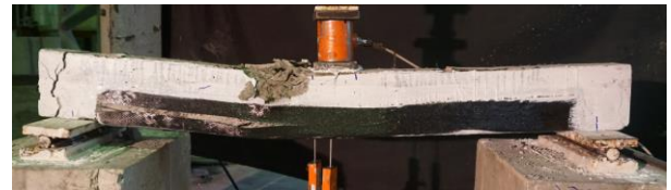
Fig. 12. Failure mode of beam BFRP-B.
