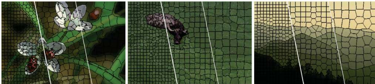
Fig. 11 Images from the Pascal Context dataset segmented by our approach with m = 20 and the number of superpixels set to 1000, 400, and 200, respectively. The resulting superpixels follow region boundaries very well.
