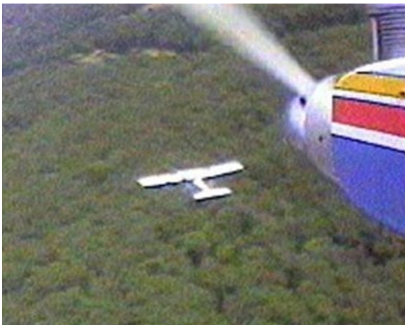
Figure 16. Aerial photo from the onboard camera during the autonomous rendezvous of two aircraft using timing control
