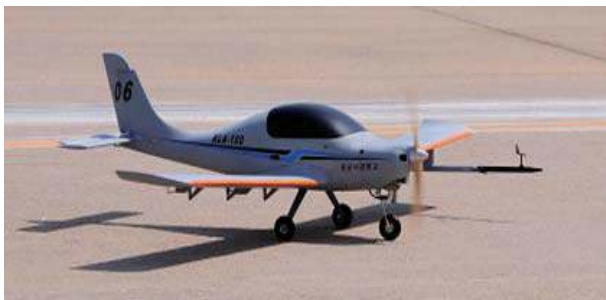
Fig. 12. Scaled RC-model of KLA-100 ready for flight tests
