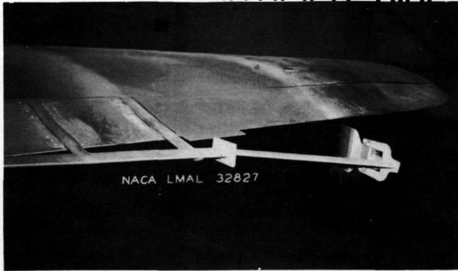
Figure 7.- Rake installation for wake surveys on right wing section. XP-47F airplane.
