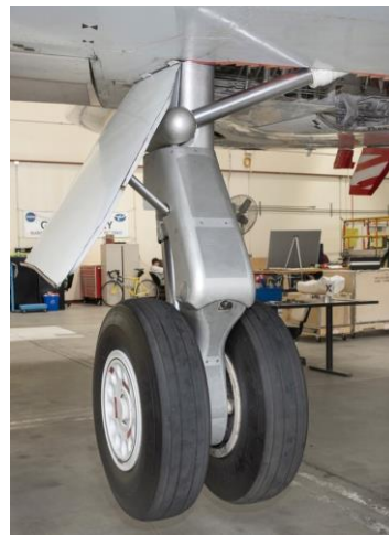
b) With fairings installed
