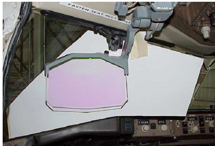
Figure 2. Vision Restriction Device in ARIES 757 aircraft.
