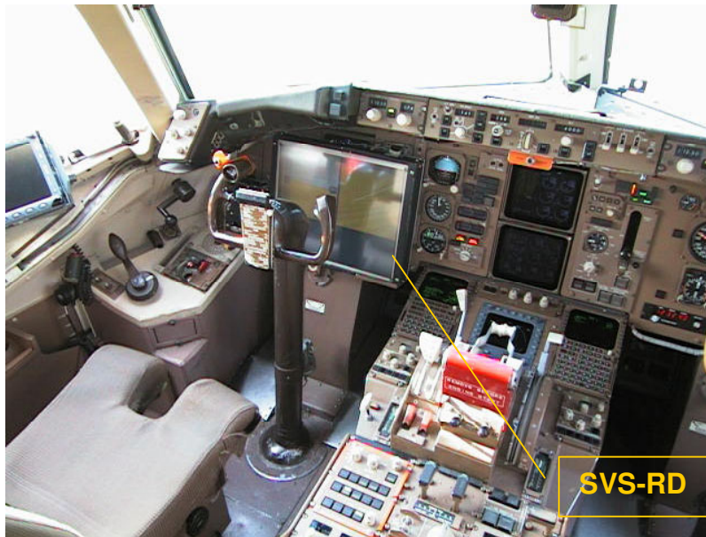
Figure 1. SVS-RD installed in ARIES 757 aircraft.
