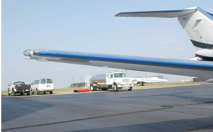
Figure 2.—Pre-activation roughness (40-grit sandpaper-blue) on wing and tails.
