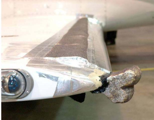
Figure 3(a).—Upper wing runback shape.
