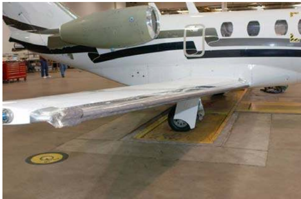
Figure 4(a).—Wing ice protection system failure case.
