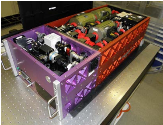
Figure 2: Transmitter: ND:YAG laser and THG.
