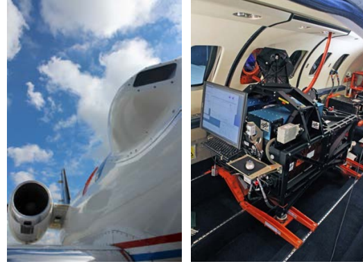
Figure 4: Left: View on the outside starboard fuselage with the fairing for laser beam transmission and reception. Right: Complete lidar and beam steering system with operator HMI.
