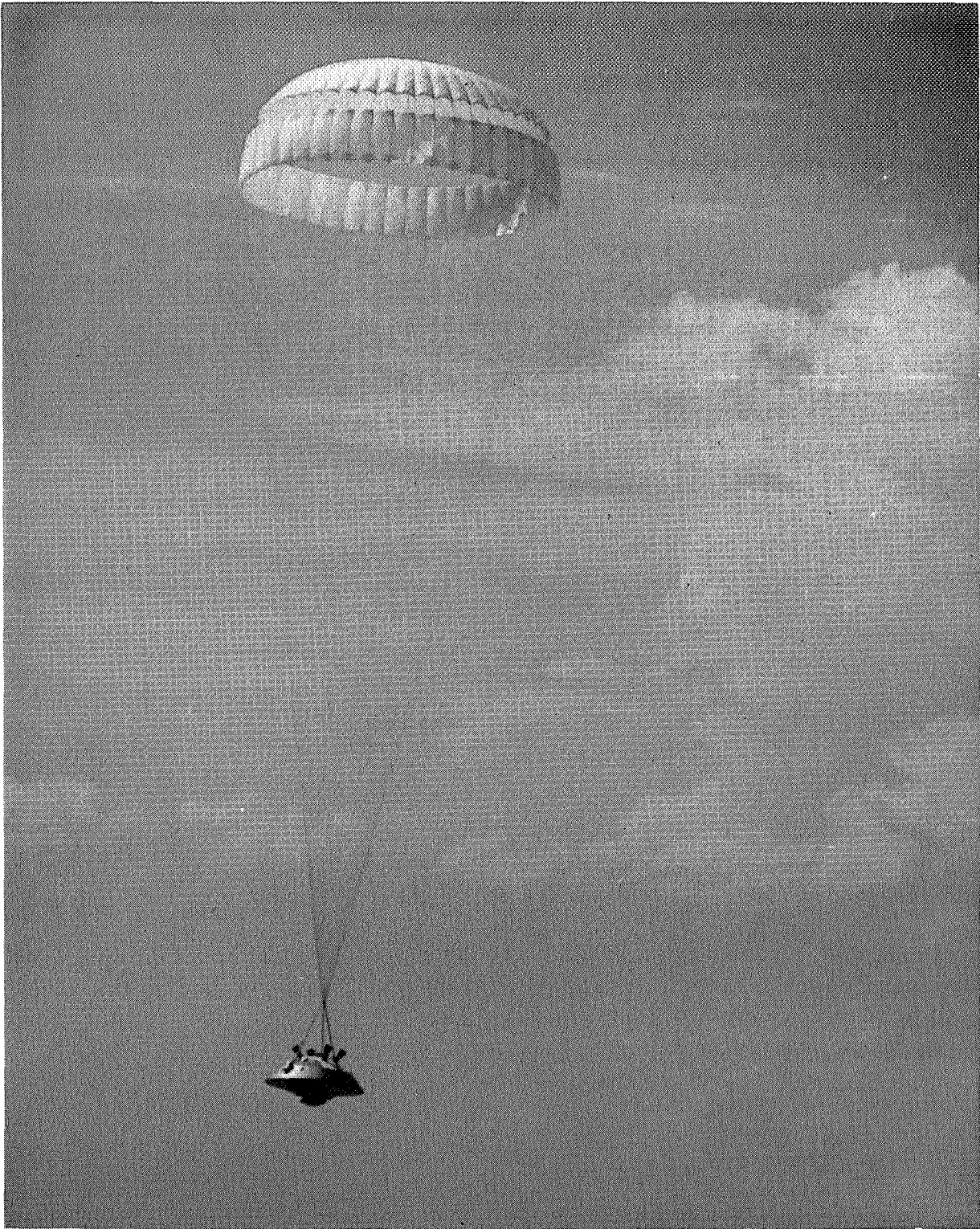
Figure 7.- Photograph of descending parachute and payload after aeroshell separation.
