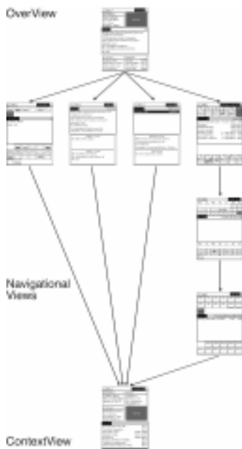
Fig. 9. Flow model of interaction with the PowerView application.
