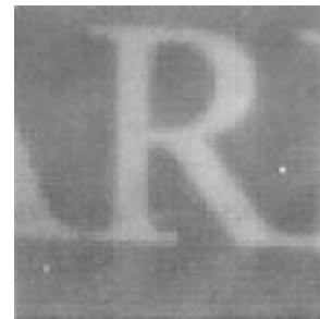
Fig. 9. Example image acquired from the adaptive imager chip after gain mismatch reduction. We projected a light-grey letter ‘‘R’’ against a dark-grey background onto the chip.
