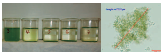
Figure 1. The effect of chitosan dose on harvesting efficiency, and floc size of Chlorella sp.
