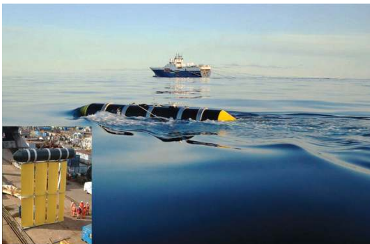
Figure 1.3: Image of a seismic vessel in operation. The float seen in the picture are holding the 'door', which provide a sideways lift to maintain streamer separation. The door is shown as an insert in the lower left corner, with some humans standing next to it.
