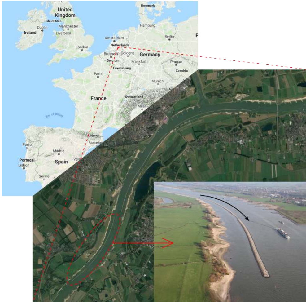
Figure 1. An overview of the LTD section in the Dutch Waal River showing the location in the Netherlands, a satellite image of the river section with LTDs (courtesy: Google) and an aerial photograph of the most downstream LTD (courtesy: Rijkswaterstaat).
