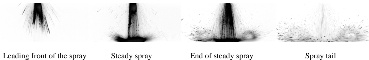
Fig. 2 – Images of spray impingement during the injection period.
