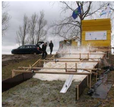
Figure 7. Test set-up with five surfboards for special measurements of flow depth, flow velocity and overtopping duration.
