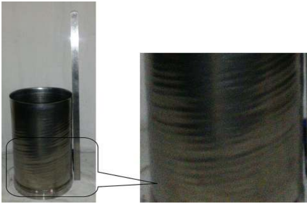
Figure 12. Flow-formed tube with vibration marks.
