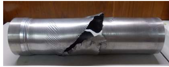
Figure 13. Surface cracks in flow formed tube.
