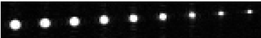
Figure 3-5. An image of the lower half of the flow phantom using a spoiled GRE sequence. The image was acquired with pixel area of 1.4 \text{ mm}^2 . The 12 lumina appear bright against a dark background on the spoiled GRE sequence.
